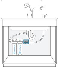
These filtration systems should be installed with a volume meter to notify you when the filters should be changed.
